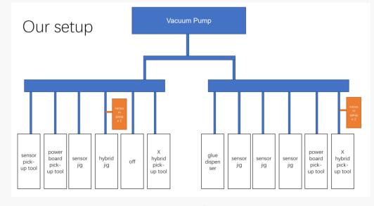
Conclusion: The vacuum of glue dispenser and powerboard pickup tool should be treated with a single vacuum pump.
