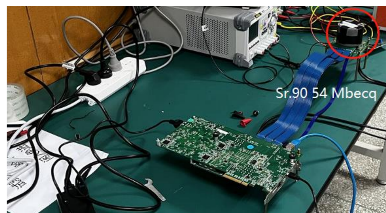
Fig. 2 A Setup of the beta source (including a DC power supply, KC705 FPGA Kit, wire bonding board, etc.)
