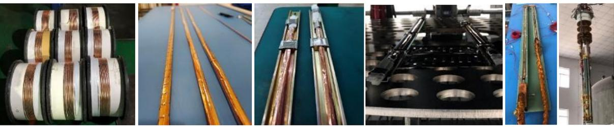
strand → cable → heat treatment → Terminal fabrication → test
