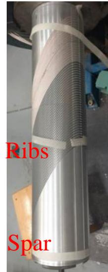
The geometry of the 4 module CCT magnet
