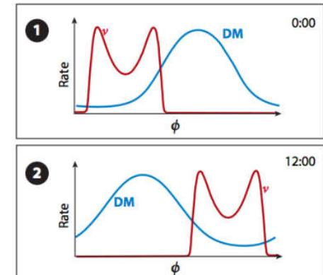
DM and solar neutrinos event rate as a function of some angle  $\phi$  on a two-dimensional readout plane at 12 h time distance or 180 degree of longitude
