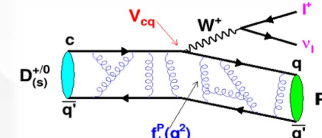
$$\frac{d\Gamma}{dq^2} = X \frac{G_F^2 |V_{cd(s)}|^2}{24\pi^3} p^3 |f_+(q^2)|^2$$
