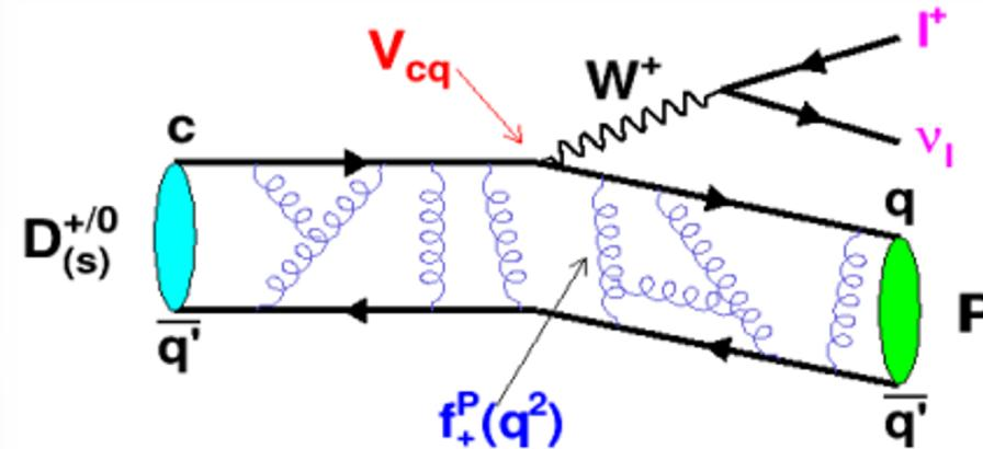
$$\frac{d\Gamma}{dq^2} = X \frac{G_F^2 |V_{cd(s)}|^2}{24\pi^3} p^3 |f_+(q^2)|^2$$
