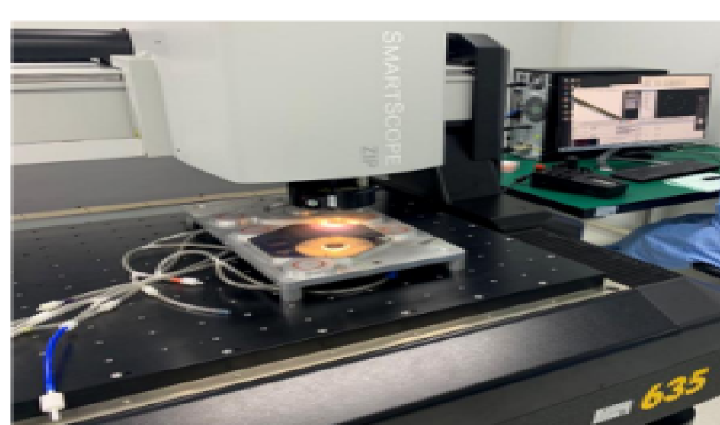
Figure 3. Checking a 8 inches silicon sensor under OGP before assembly into a module.
