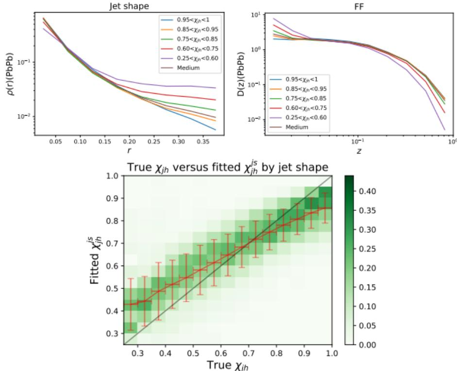
$$\chi_{jh}^{is} = \sum_i \left( \frac{\rho_{Ti}}{\rho_T} \right)^{\alpha_i} r_i^{\beta_i} + \gamma$$
