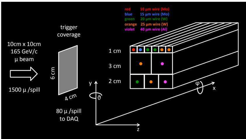
The test was performed during November 2021 at CERN on the H8 beam line in a **parasitic mode**. Main users on the same beam line was a team testing a tile calorimeter and, therefore, requesting for **large part of the time, beams of electrons and hadrons, at various energies, needed for their calibration, but useless for our purposes**. Only **sporadically**, a beam of **165 GeV/c muons** was available for us.
