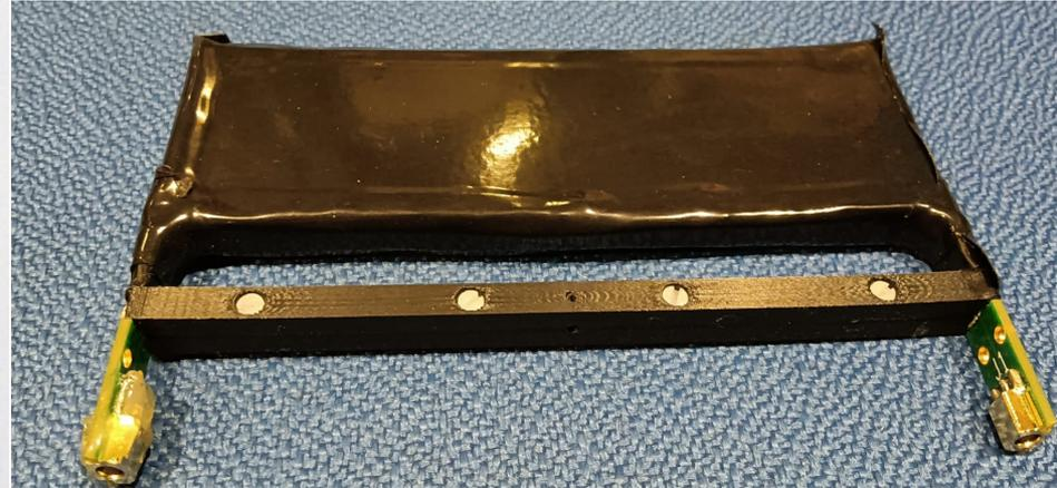
12cm x 6cm upstream and downstream scintillator tiles (designed and used as timing counter of the MEG2 experiment at PSI) used in coincidence and readout by SiPM
