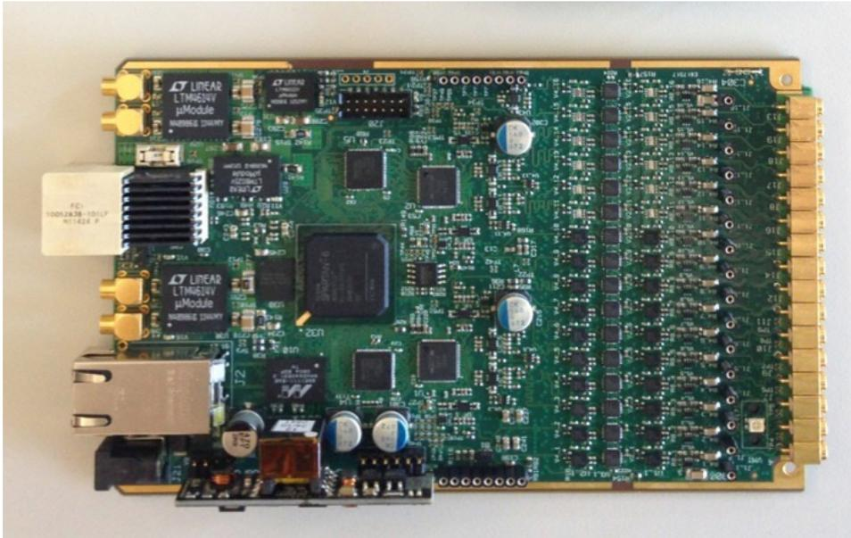
16 channels data acquisition board designed and used by the MEG2 experiment at PSI ( $\mu \rightarrow e + \gamma$ ) (credit to S. Ritt, Paul Sherrer Institute, Zurich, Switzerland)
