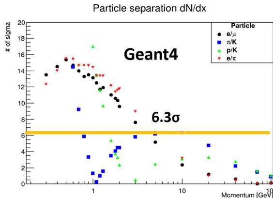
Despite Geant4 uses the cluster density and the cluster size distributions from Garfield++, it disagrees from Garfield++ and, therefore, from the analytical calculations also.
