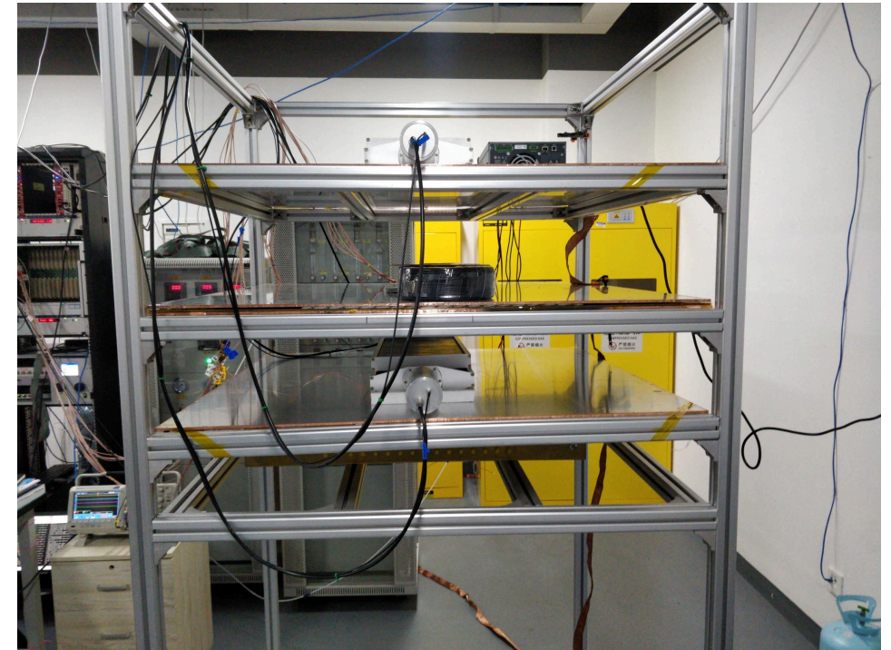
Cosmic muons test setup
