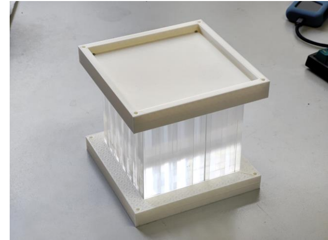
A dummy crystal matrix with 3D printed support structure
