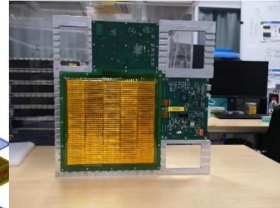
ScECAL prototype with 6700 channels
