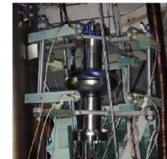
Second sound cavity quench detection system
