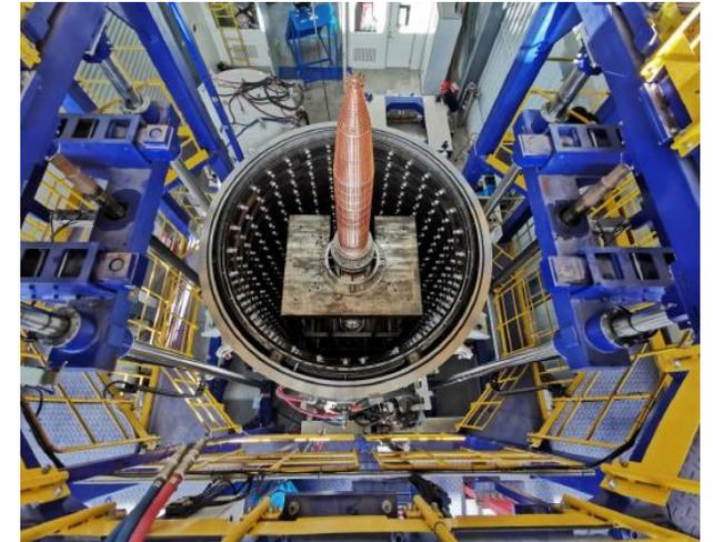
The 2<sup>nd</sup> Klystron (under test)
