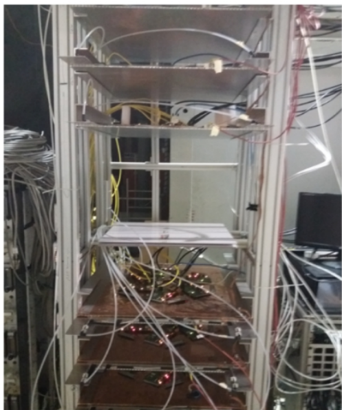
Setup with 8 detectors equipped with the new readout scheme Large PCB
