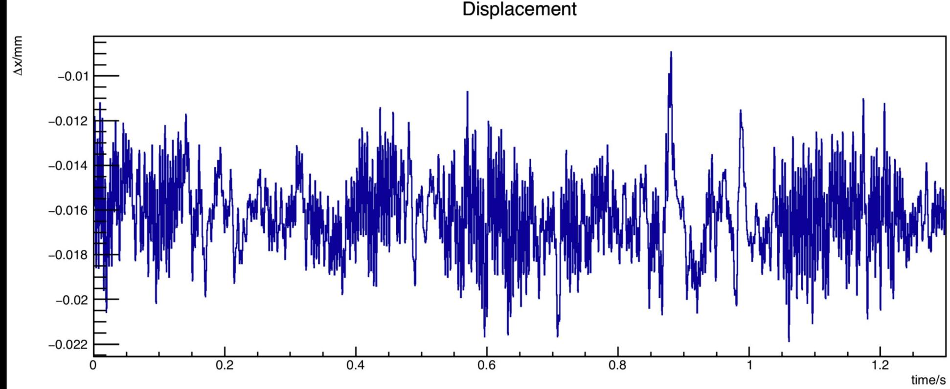
Typical Vibration displacement during air cooling
