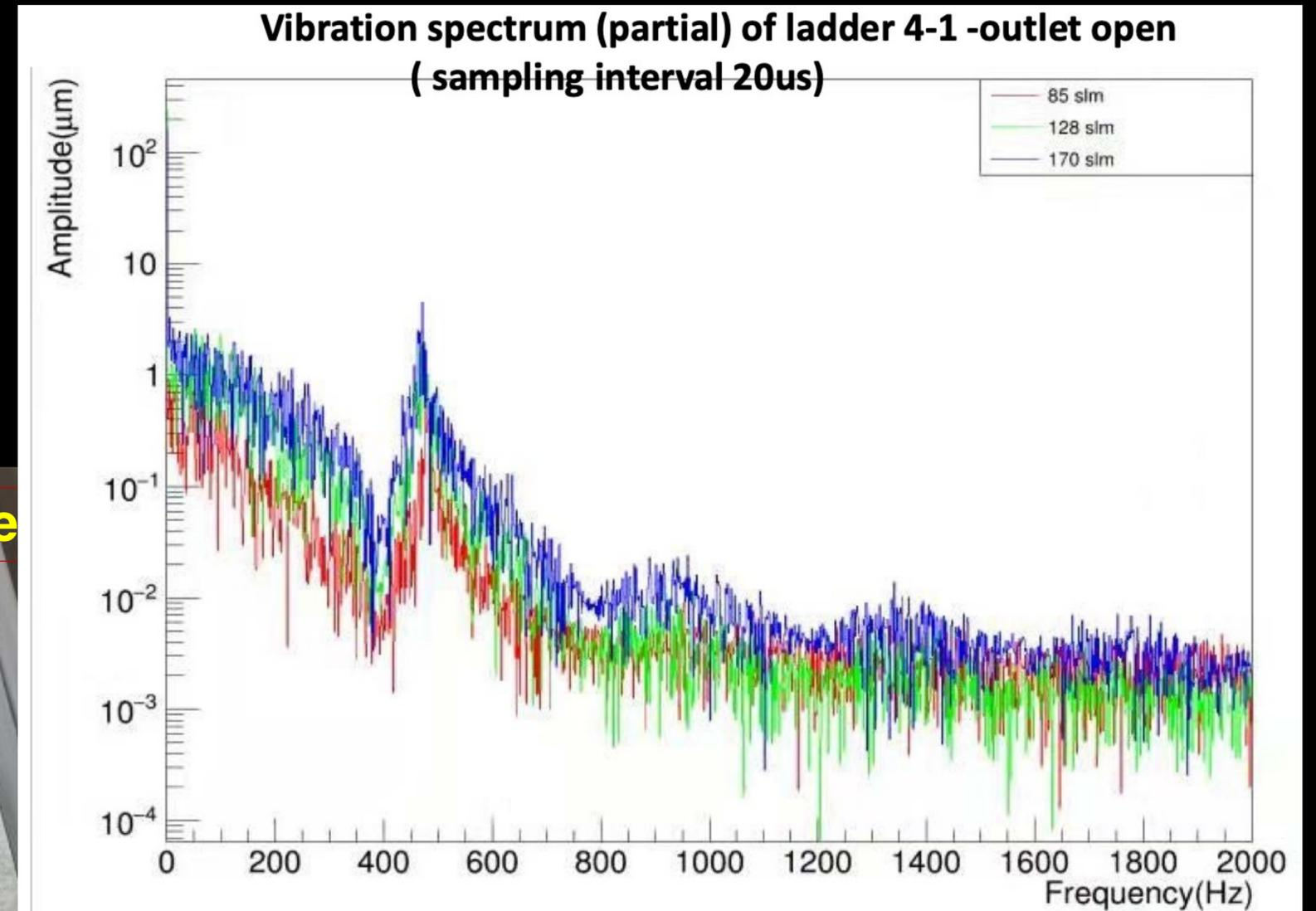
A few resonant peaks were confirmed at frequencies below 2000 Hz.
