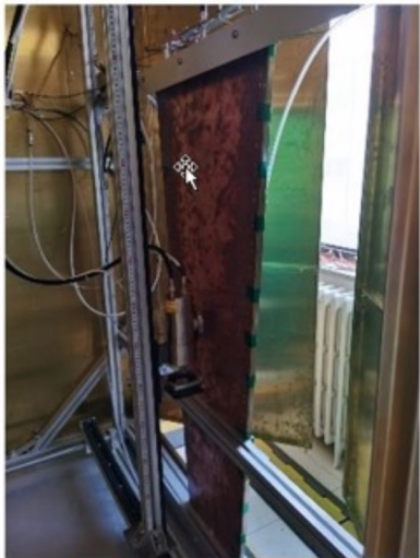
GEM X ray gain test at PKU
