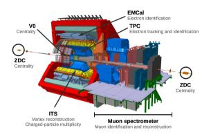
p–Pb and Pb–Pb: Muons reconstructed in the forward spectrometer  $(-4<\eta<-2.5).$  Probing of the low  $(\sim 10^{-4}$  to  $\sim 10^{-3})$  and high  $(\sim 10^{-1}$  to almost unity) Bjorken-x regions.
