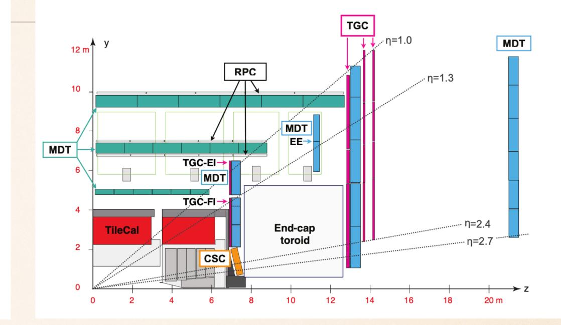
The ATLAS detector consists of an inner tracking detector, calorimeters and a muon spectrometer, which provides precision combined muon
