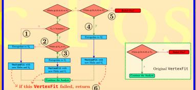
Therefore, we developed a more sophiscated algorithm and take every detail into consideration to correct both the materials' effect and magnetic field effect. We combine the traditional vertex fitting algorithm, Kalman filtering method, and intelligently choosing the default helix together into a well designed flow chart to cover all the cases in the analysis.
