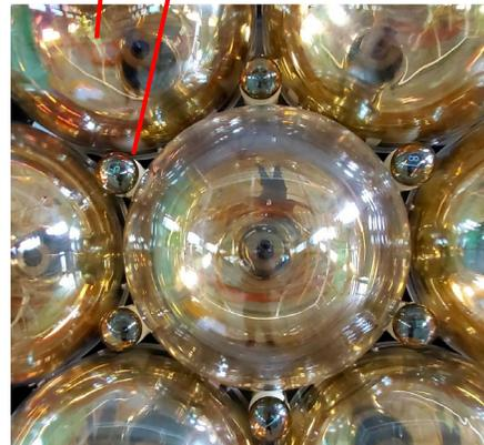
The PMT system acts like a “dual camera system”, which is able to capture the temporal evolution signals originated from neutrino.
