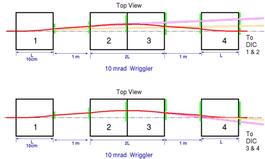
**Figure 5:** (Top - Bottom): A. Schematic diagram showing the location of collimators (yellow strips) on the wiggler pole faces which guide the SR photons produced at the wiggler magnet to the beam left ionization chamber.; B. Schematic diagram showing the location of collimators on the wiggler pole faces which guide the SR photons produced at the wiggler magnet to the beam right ionization chamber.
