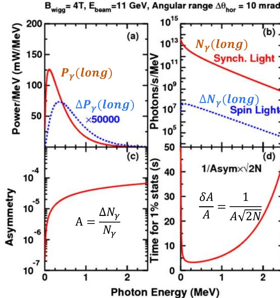
(b) The number of SR photons  $N_\gamma$ , and the spin-light photons  $\Delta N_\gamma$
