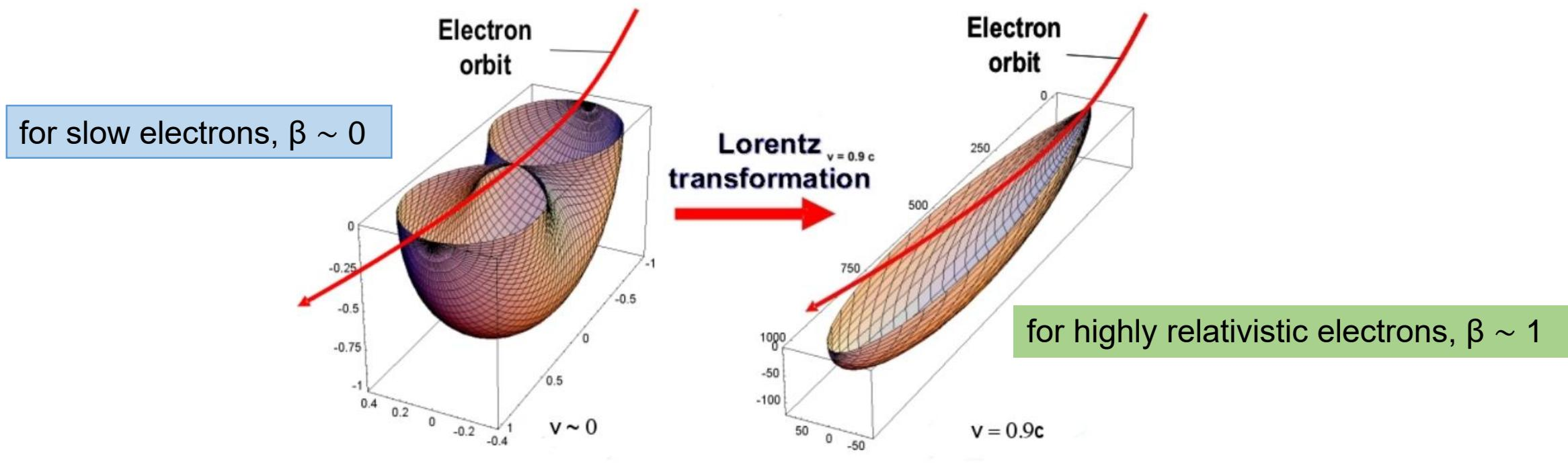
Angular distribution of synchrotron radiation shown for the bottom half of the electron's orbital plane.
