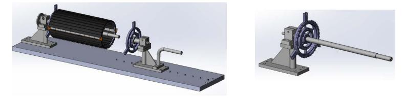
The cantilevered *outer barrel* on tooling sinks: (273/120) x 0.019= 0.04mm
