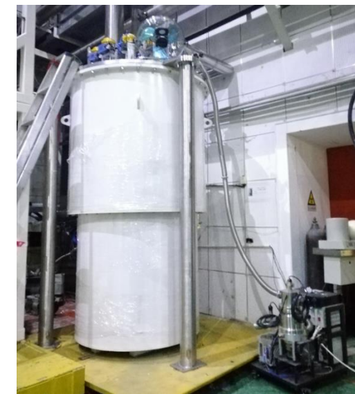
Photo of test cryostat
