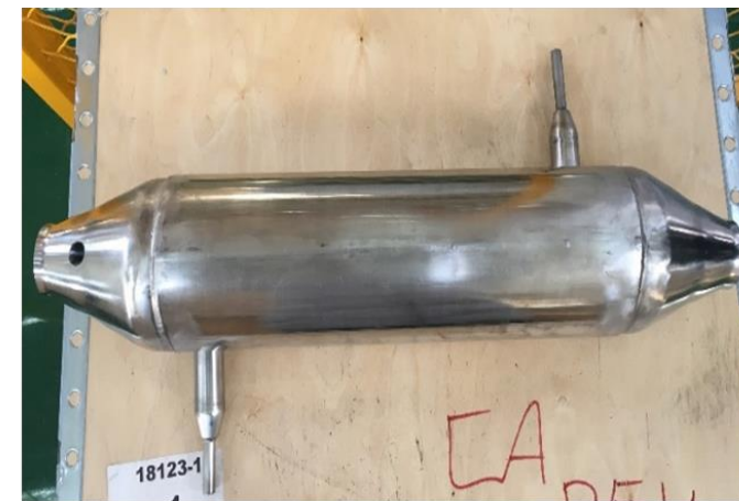
Photo of the manufactured Single Layer Coiled Finned-tube HX
