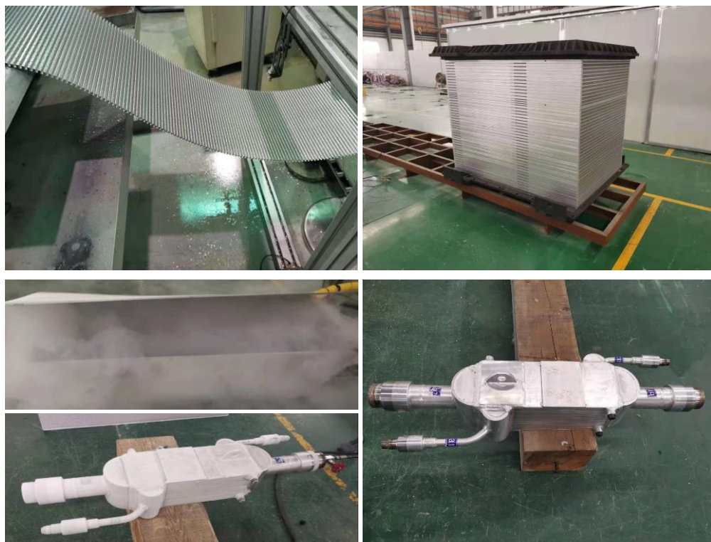
Manufacture process of Plate Fin HX
