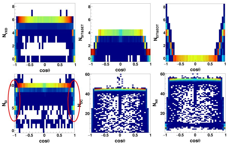
■ Barel: ~10 silicon hits used in fit; Endcap: 10 or less, determined by vertex cover range
