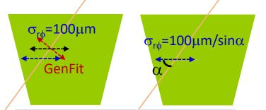
With ratio: close contribution in fit  $\frac{(r\phi - r\phi_{extra})}{\sigma_{r\phi}} \approx \frac{\left(L_{drift} - L_{drift,extra}\right)}{\sigma_{L}}$
