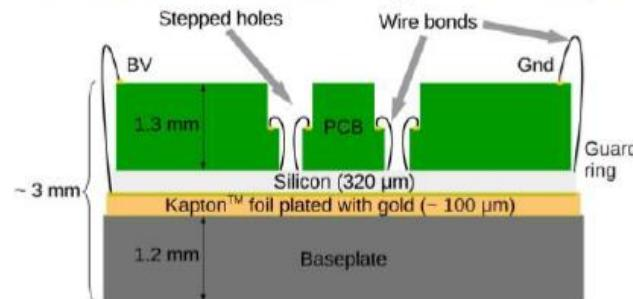
➤ Wire-bonding quality (by pull tester): wire-bonds can fulfill the strength requirement
