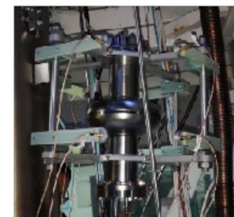
Second sound cavity quench detection system
