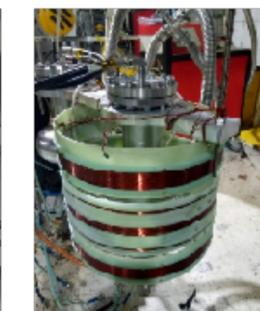
Helmholtz coil for cavity vertical test
