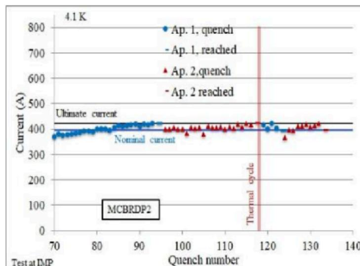
➤ Full size prototype magnet MCBRDP2 was completed in May, 2020. Both apertures reached the ultimate current.
