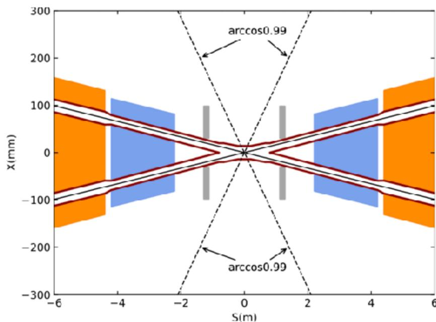
Final focusing magnets (QD0, QF1) with Segmented Anti-Solenoidal Magnets
