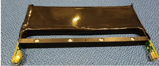
**Two scintillator tiles** (12 cm x 4 cm), placed **upstream** and **downstream** of the drift tubes pack, instrumented with SiPM.
