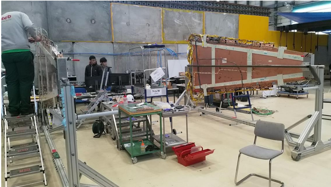
8) An installed chamber undergoing system tests: electronics, cooling and gas.
