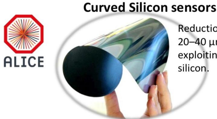
Reduction of thickness to about 20–40  $\mu\text{m}$  open possibility of exploiting the flexible nature of silicon.
