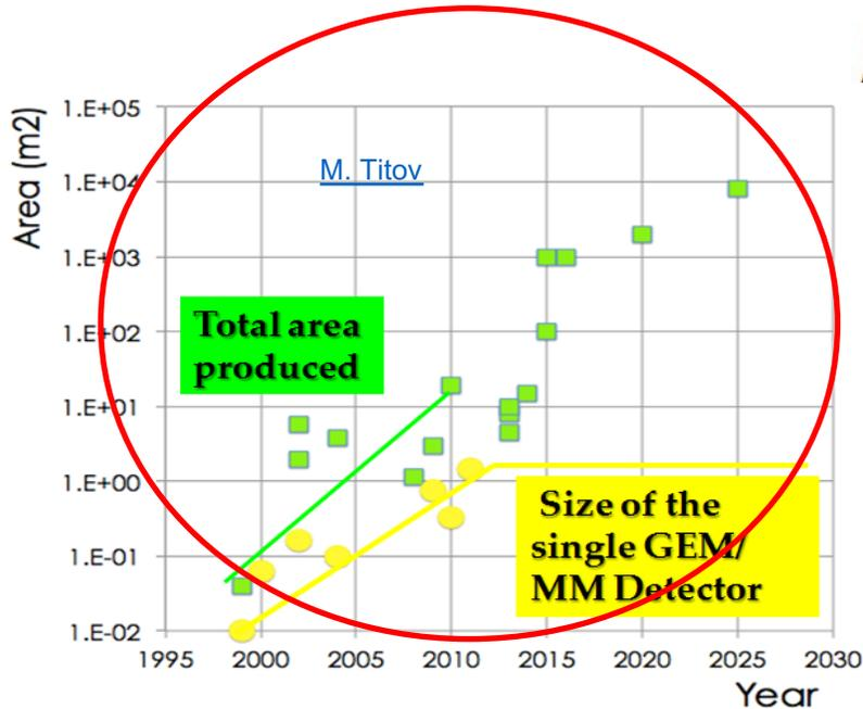
From widely used MWPC to widely used MPGD has taken 50 years
