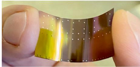
50 $\mu\text{m}$  pixel, waferscale
