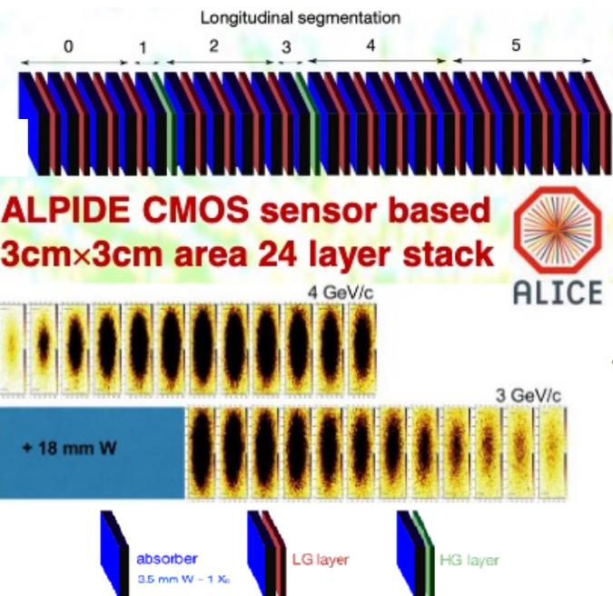
**DRDT 6.1:** The enhanced electromagnetic energy and timing resolution most relevant in next decade for upgrades of ALICE and LHCb.
