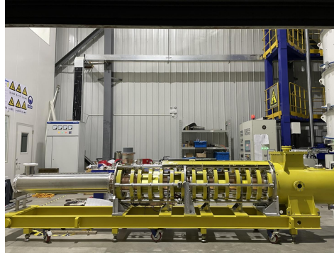
Klystron No. 2 Efficiency 77% (2021)
