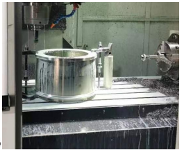
Klystron No. 3 (MBK) Efficiency 80.5% (under fabrication)
