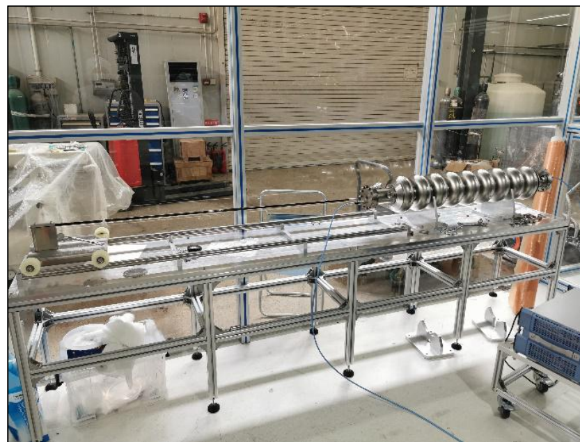
RF field measurement (in cleanroom)
