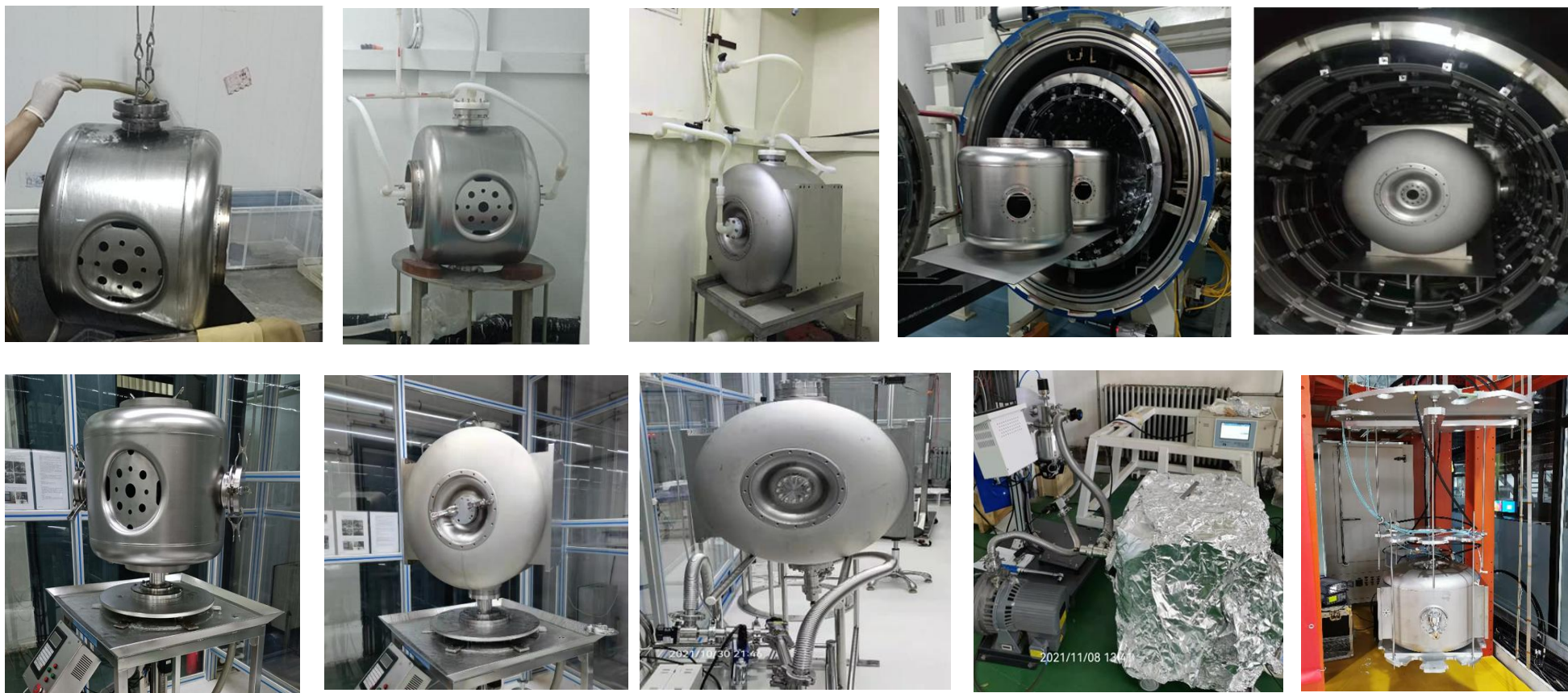
Cavities for SSR2 (RISP project of SSR2)
