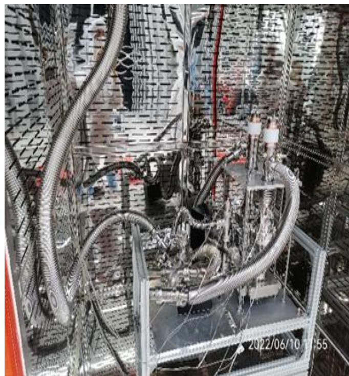
Leak test, baking and conditioning (PAPS)
