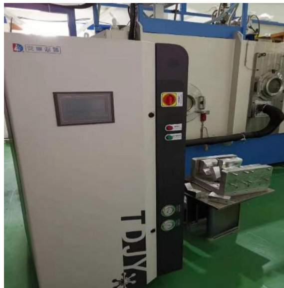
Cold Trap and Fast Cooling System for EBW Machine
