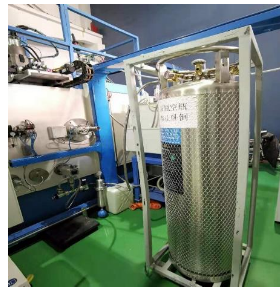
Cold Trap and Fast Cooling System for EBW Machine
