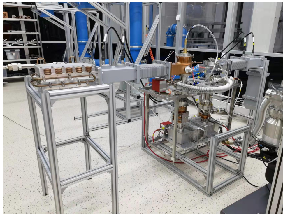
Leak test, baking and conditioning (PAPS)
