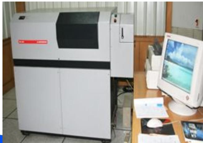
全谱直读光谱仪 ICP full spectrum direct reading spectrometer
