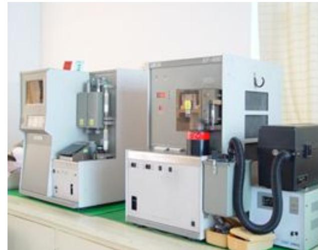
氧-氮量仪 TC-600 oxygen-nitrogen analyzer
