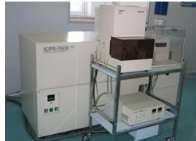
光谱仪 ICP-AES spectrometer
