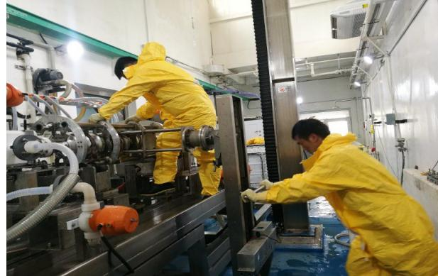
EP for 1.3GHZ-9cell cavity
