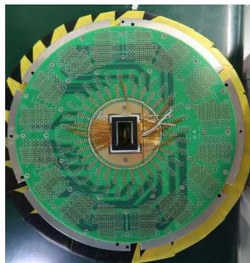
Probe card for wafer test
