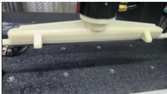
Dummy ladder glue automatic dispensing using gantry
