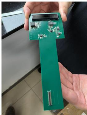
Ladder readout in vertex detector mockup
