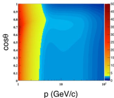
PID evaluation with  $K^\pm$  identification,  $D^0 \rightarrow \pi^+ K^-$  and  $\phi \rightarrow K^+ K^-$  reconstruction based on the full simulation of  $Z \rightarrow q\bar{q}$  samples.
