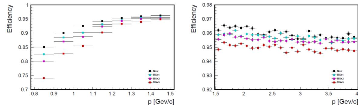
Figure 4: Muon identification efficiency after the requirement  $\text{muonID} > 0.9$  in the three considered scenarios for tracks with  $0.8 < p < 1.5 \text{ GeV}/c$  (on the left) and for tracks with  $1.5 < p < 4.9 \text{ GeV}/c$  (on the right).
