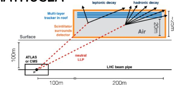
**Fig. 1:** Simplified detector layout showing the position of the  $200\text{ m} \times 200\text{ m} \times 20\text{ m}$  LLP decay volume used for physics studies. The tracking planes in the roof detect charged particles, allowing for the reconstruction of displaced vertices in the air-filled decay volume. The scintillator surrounding the volume provides vetoing capability against charged particles entering the detector.
