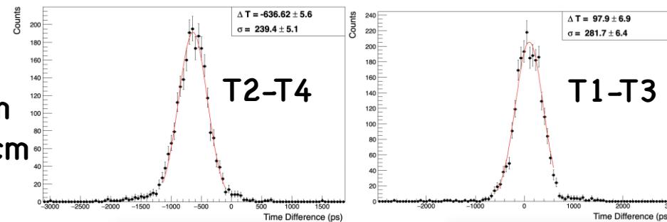
➤ Caused by photon propagation&& cosmic ray angle effect
