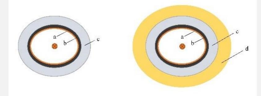
In IW2D a:2  $\mu$ m TiN, b: 5 mm Ceramic chamber, c:5 mm Air, d:PEC
