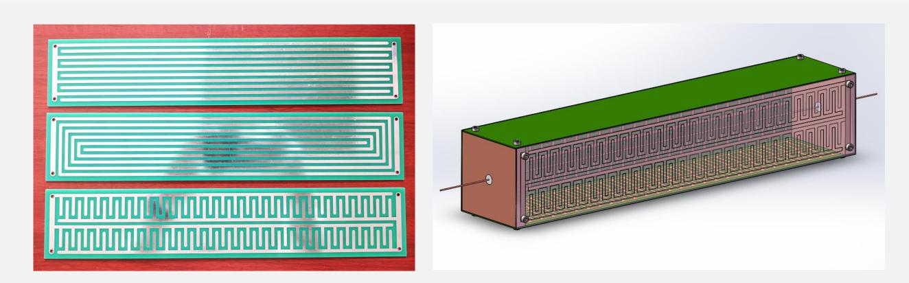
The coating patterns printed on PCBs and the concept design of testing transmission characteristics by coaxial line . (The Figure Above)
