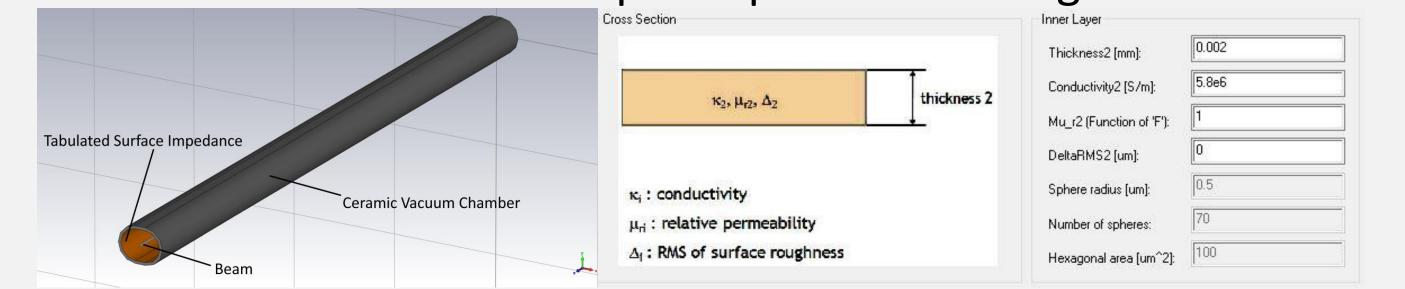
The longitudinal impedance of the uniform coating is 1  $\Omega$  or less. The transverse impedance converges at a wake length of about 50 m, and the results are similar to IW2D. More results are being calculated.....
