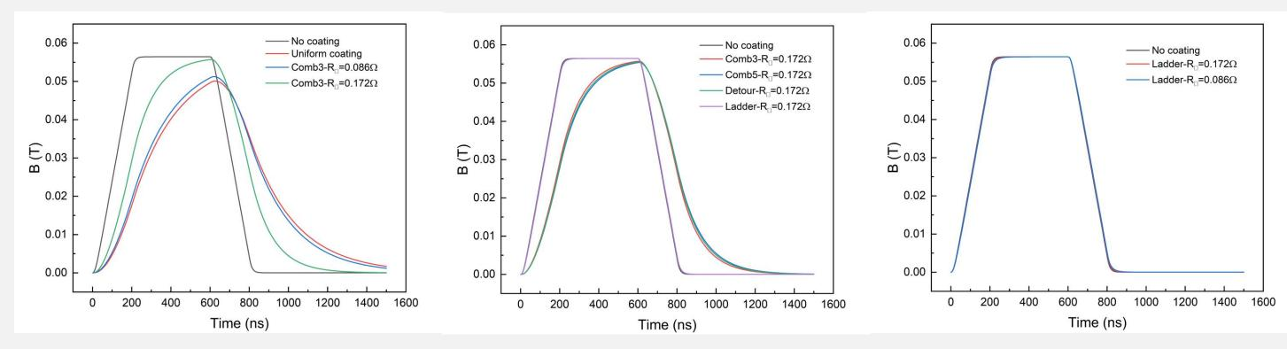
Comb and detour-shaped pattern coatings are **incapable** of maintaining magnetic field waveform, even if the film's square resistance is increased.
