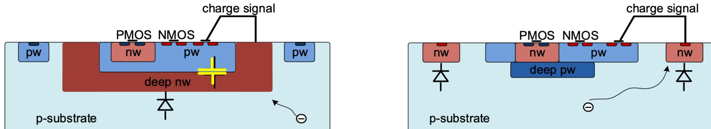
Fig. 4: The schematic of HV-CMOS (left) and LV-CMOS (right)
