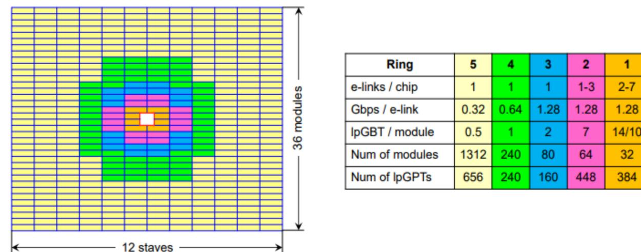
Fig. 7: The IpGBT allocation and configuration plan.
