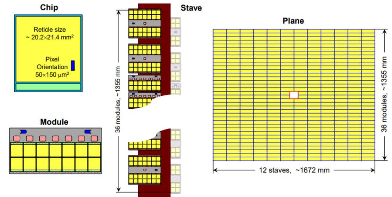
Fig. 5: A possible configuration for the Upgrade II UT detector.
