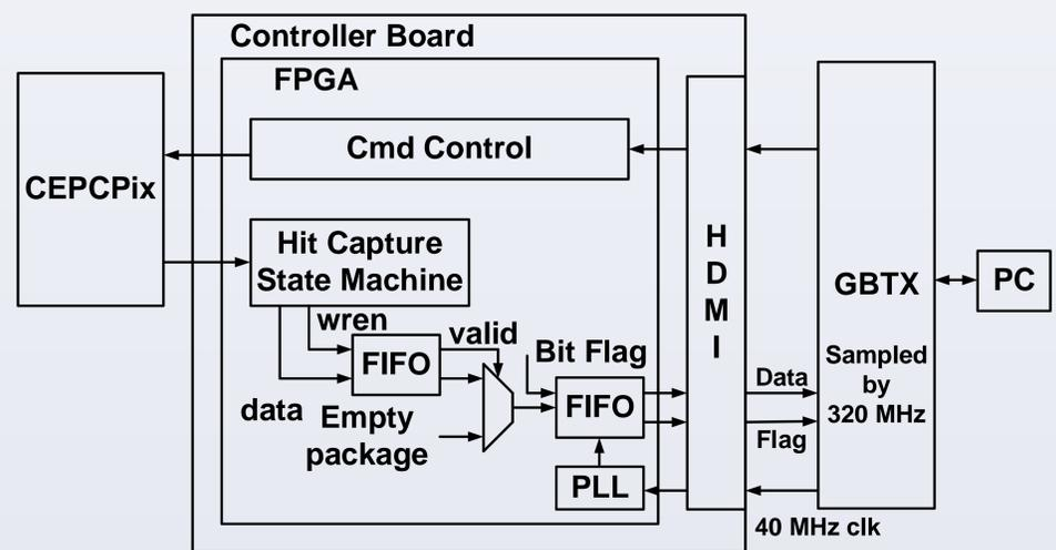
Fig. 2. DAQ hardware for CEPCPix
