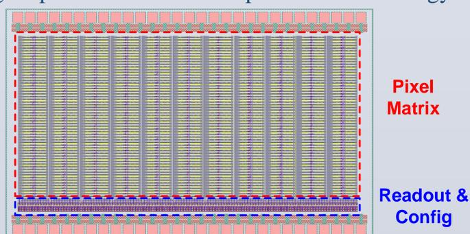
Fig. 1. Prototype layout of CEPCPix
