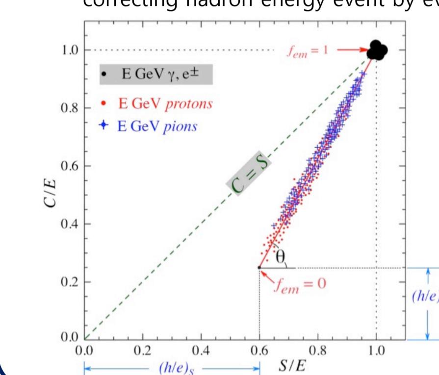
$$\begin{aligned} 1. C &= E \left[ f_{EM} + \frac{1}{(e/h)_c} (1 - f_{EM}) \right] \\ 2. S &= E \left[ f_{EM} + \frac{1}{(e/h)_S} (1 - f_{EM}) \right] \\ 3. f_{EM} &= \frac{(h/e)_C - (C/S)(h/e)_c}{(C/S)[1 - (h/e)_S] - [1 - (h/e)_c]} \\ 4. x &\equiv \cot \theta = \frac{1 - (h/e)_S}{1 - (h/e)_c} \\ 5. E &= \frac{S - xC}{1 - x} \end{aligned}$$
