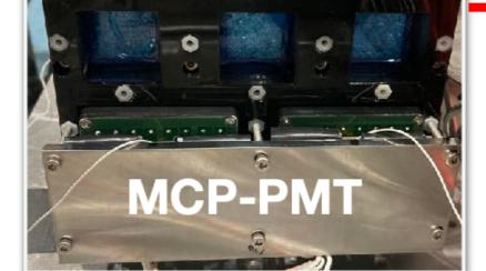
We stacked the PMTs layer by layer to compose the readout system
