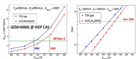
Figure 1: The IBF x Gain as a function of  $V_{GEM}$ (Left), and the Gain as a function of  $V_{GEM}$ (Right)
