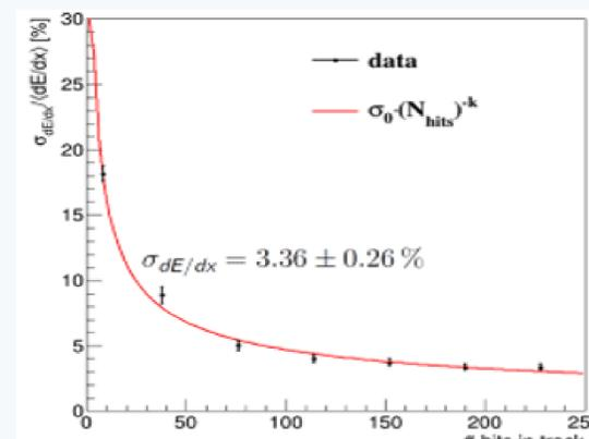
Figure 5: The dE/dx resolution versus the number of hits in a pseudo-track of various length
