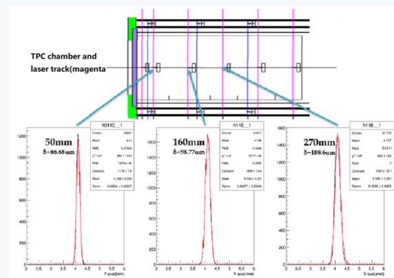
Figure 4: Spatial resolution at different drift length
