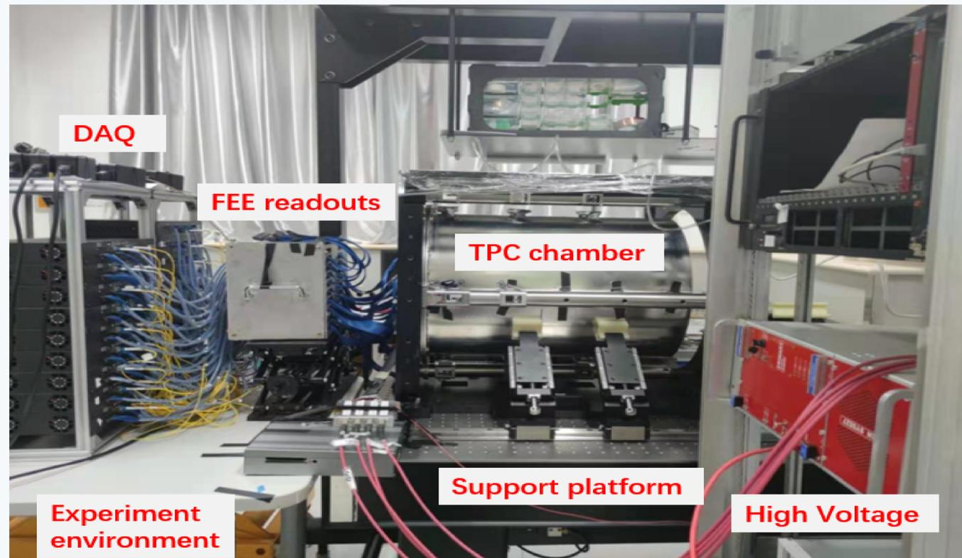
Figure 3: TPC prototype with integrated 266nm UV laser
