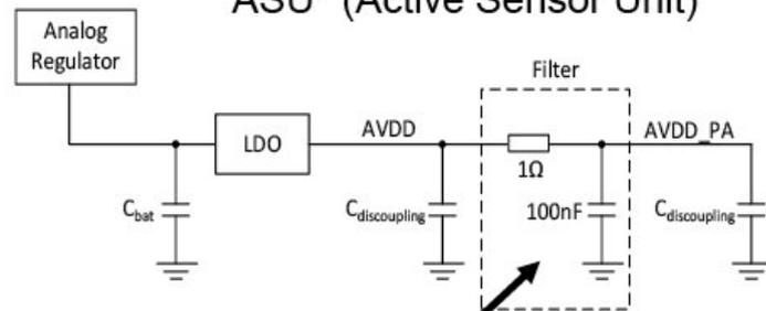
Add filter to generate local preamplifier power supply
