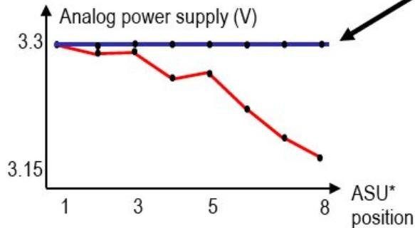
In the electrical long SLAB, 8 boards are chained and due to resistivity of layer per board on analog 3.3V, we measure voltage drop along the long SLAB coupled with bandgap distribution.
