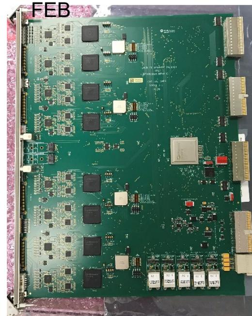
→ Each FEB receives clock, commands and configuration from 3CU (backplane) and provides data on 4 optical links (mono-dir) to TELL40
