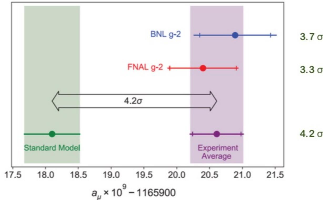
$$a_\mu^{\text{EXP}} = (116592089 \pm 63) \times 10^{-11} [0.54 \text{ ppm}] \quad \text{BNL E821}$$
