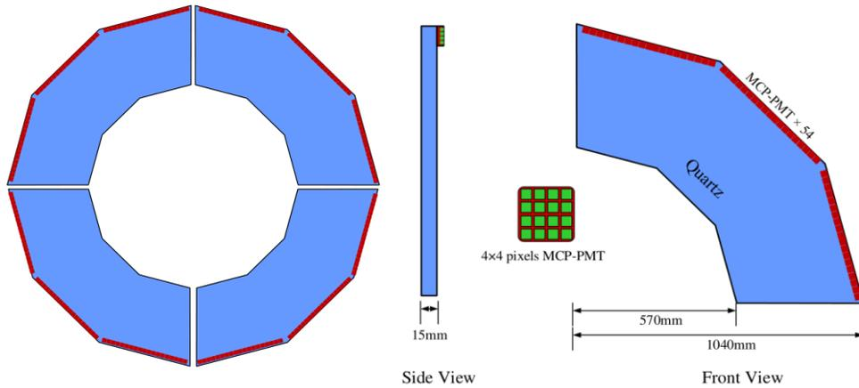
Detection of Internal total-Reflected Cherenkov light (DIRC)
