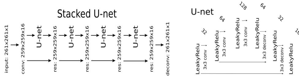
FIG. 1: An illustration of the encode-decode network, **stacked U-net**, which consists of the input and out layers and four residual U-net blocks. The right figure shows the U-net structure, and the depth of the hidden layer is written on the top of them.
