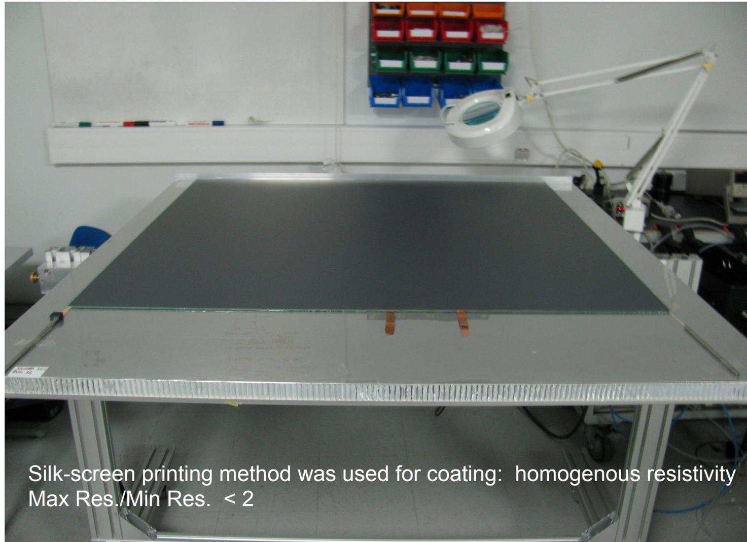
Silk-screen printing method was used for coating: homogenous resistivity
