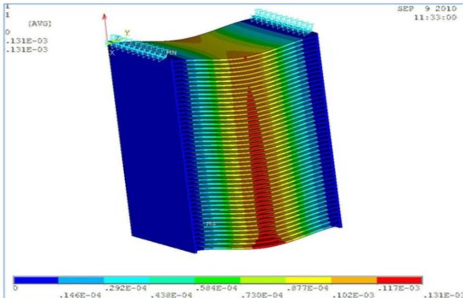
Maximum deformation was found To occur during manipulation (rotation, transport) but still with no effect on the cassettes. A rotation tool will allow to use the prototype to study cosmic rays... tests will be conducted during assembling to check this possibility.
