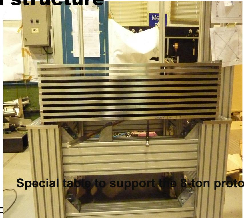
**Special table to support the 8-ton prototype**
