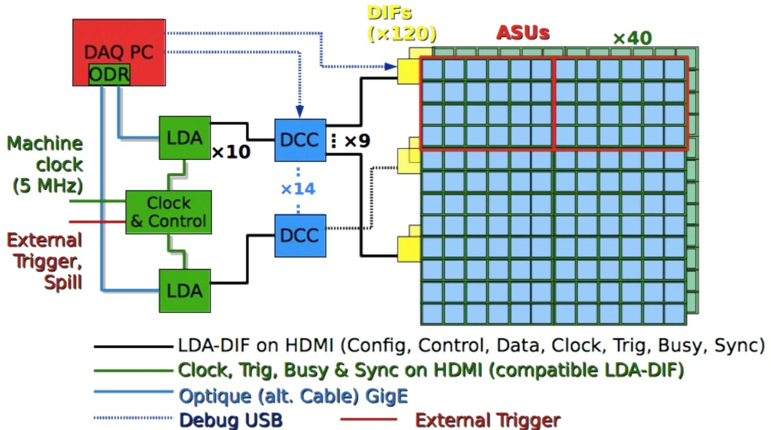
The full chain of the new generation of CALICE DAQ was successfully tested
