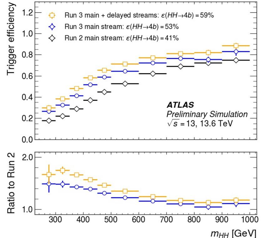
The asymmetric 4-jet trigger in Run 3 increase the SM  $HH \rightarrow 4b$  signal efficiency from 41% to 59%.
