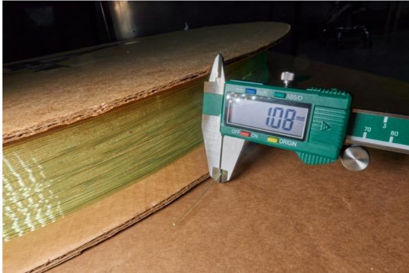
Saint-Gobain WLS Fiber 1.0mm Dia.
