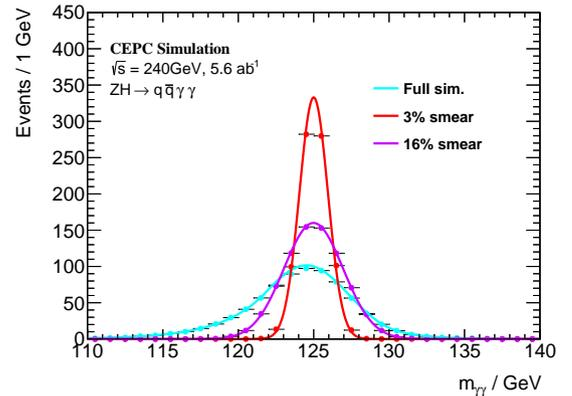
**Figure 5:** The signal shape for the full simulated  $H \rightarrow \gamma\gamma$  sample (blue) and for two samples with smeared photon energy (3% in red and 16% in violet). The fitted signal width are 2.81 GeV, 0.94 GeV and 1.96 GeV respectively.
