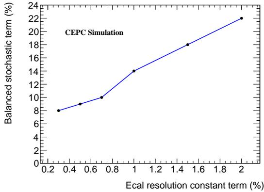
**Figure 7:** The balanced ECAL stochastic resolution points with different configurations of the constant term.
