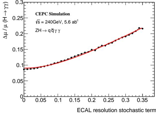
**Figure 6:** The  $Br(H \rightarrow \gamma\gamma)$  precision in  $ZH \rightarrow q\bar{q}\gamma\gamma$  channel as a function of the stochastic term in ECAL resolution from a fast analysis. The points are fitted with Eq. 5.
