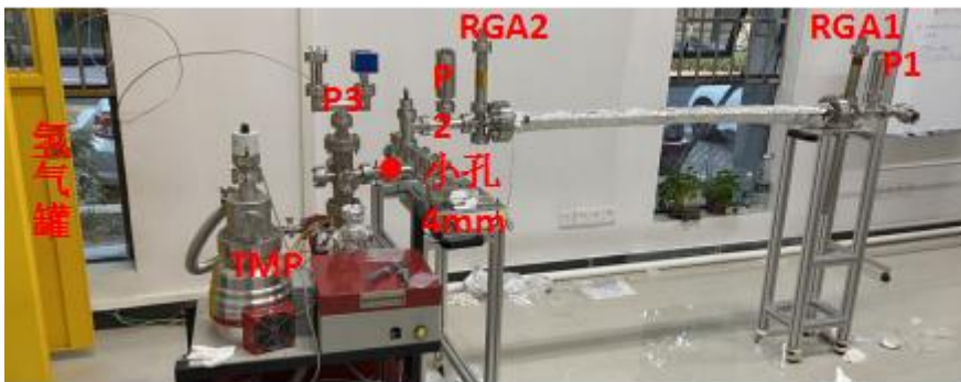
6 m vacuum pipe have been installed on the NEG coating setup
