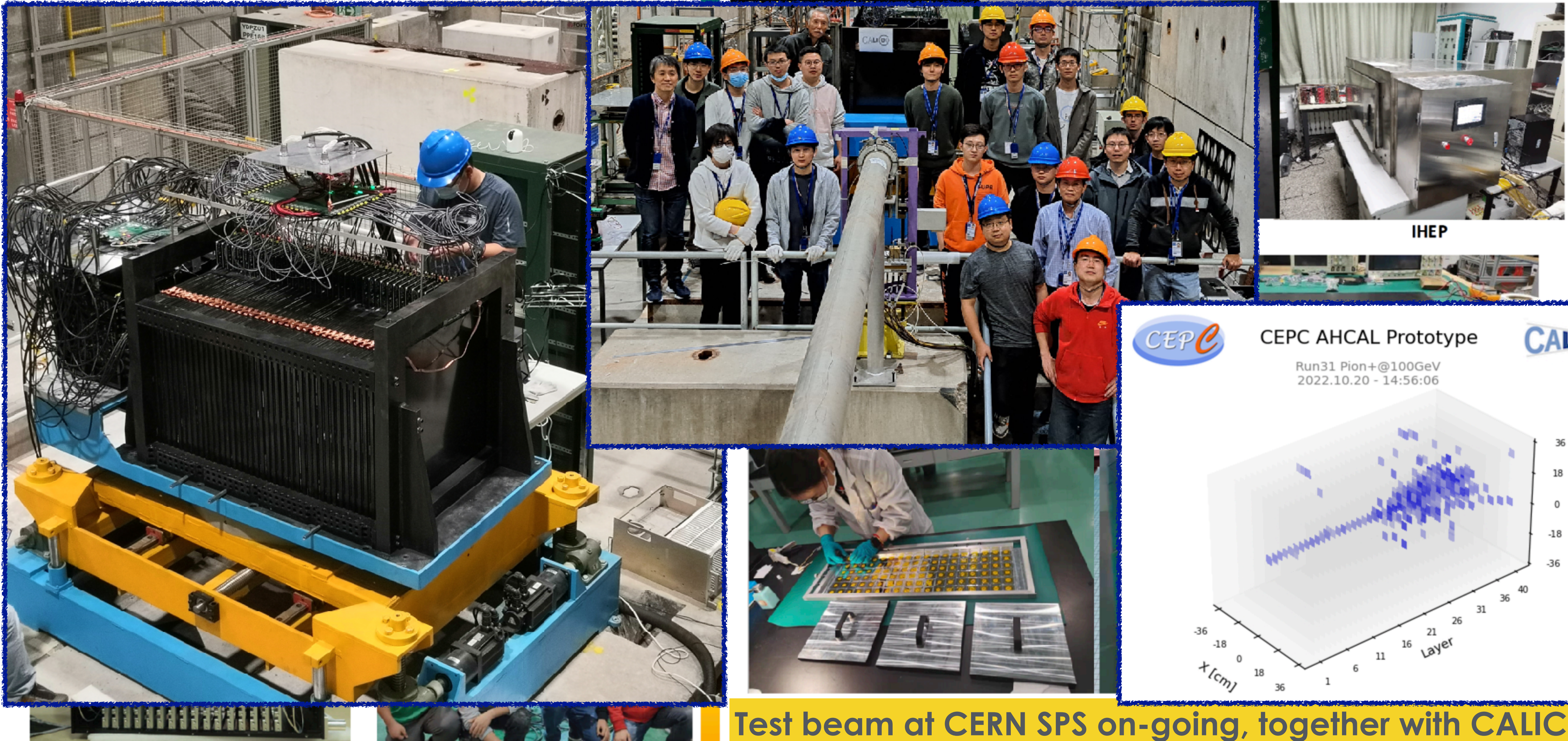
Combined ScW-ECAL and AHCAL test beam
